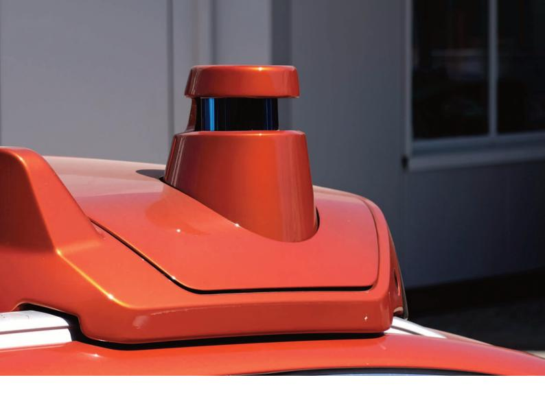
iDAR is among the key sensor technologies underpinning the automotive industry's quest to make fully autonomous vehicles (AVs) a reality. Capable of creating 3D digital representations of a vehicle's environment, LiDAR is invaluable for obstacle detection and safe navigation.
